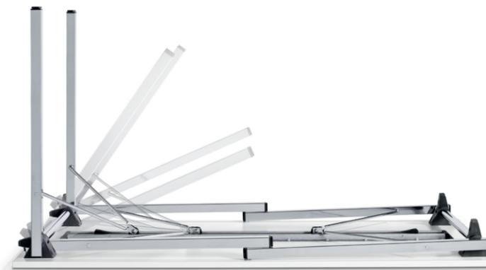
The folding mechanism works in the same way for both T-leg and four-leg tables. There are no controls to unfold the tables, which lock in place automatically. Pressing a button releases the locking device, ready for folding. Sturdy plastic pads protect the surface of the table and prevent it being damaged when the tables are stacked. There are special trolleys to carry the stacked tables efficiently.
